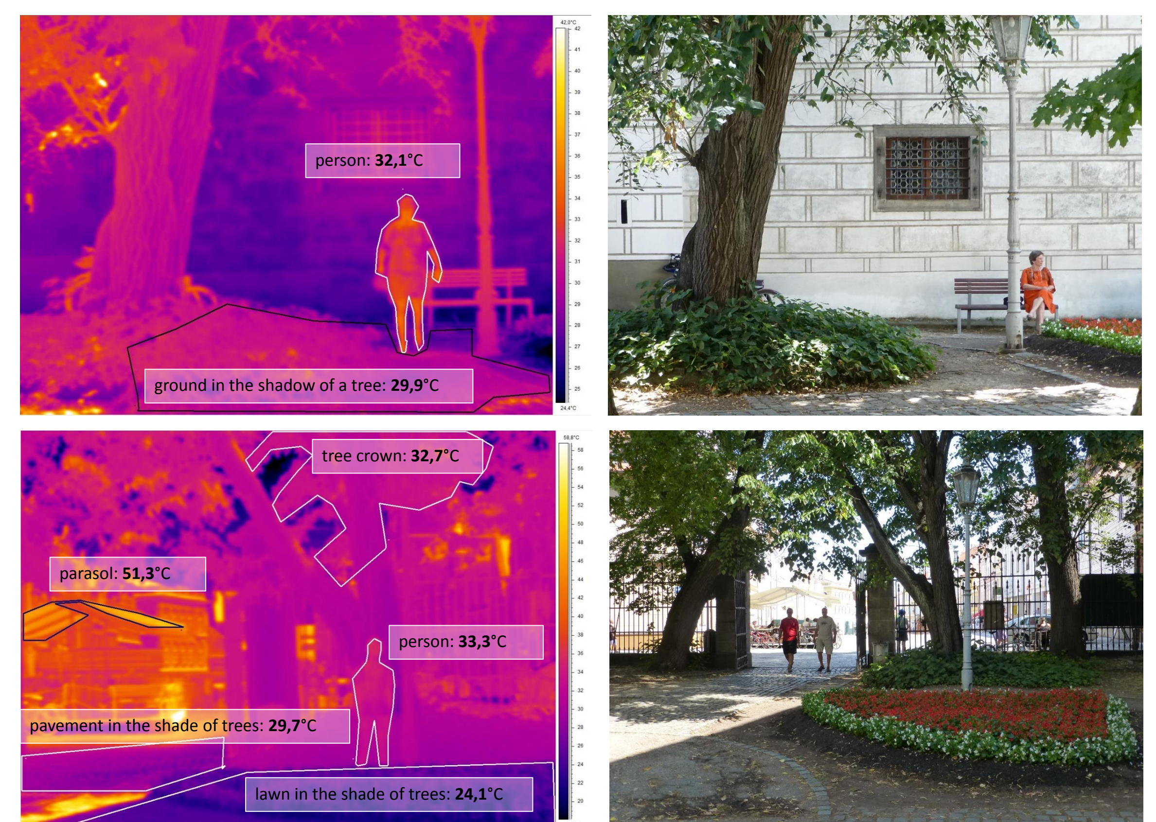
Fig. 3. A parasol over a person in a restaurant has a temperature of 51,3^\circ\text{C} while the temperature of the tree crown is only 32,7^\circ\text{C} . The area under the parasol is still quite hot, reaching a temperature of 36,3^\circ\text{C} (see also Fig. 2), whereas the lawn in the park has only 24,1^\circ\text{C} .
